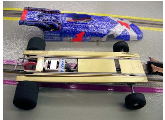
Wes' car: Samson chassis, 114.8 grams, Fast Ones ProSlot, OS Cooper, 7/28, JK Guide, JK Treated Rears, JK Fronts, Difalco HD 30 Controller.
