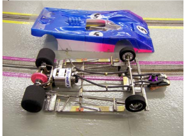
Jay's car: Tony P Triagra chassis, ProSlot, OS TI22, 8/30, Parma Guide, JK Treated Rears, Cyr / Mac Fronts, 3 rd Eye Controller
