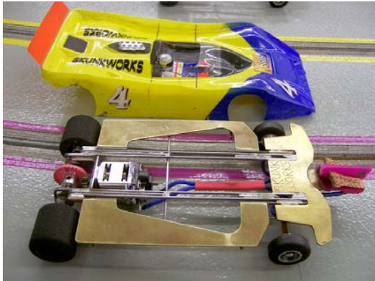
Matt's car: Tony P Project X chassis, ProSlot, OS TI22, 8/29, JK Guide, JK Treated Rears, Sonic / Bruce Fronts, 3 rd Eye Controller
