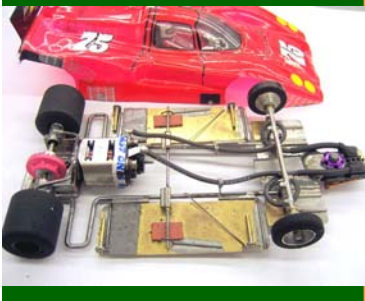
The Winning Car Tony P Twistamon frame, 119.5 grams, OS Chevron GT, Fast Ones ProSlot, 7/27, Red Fox Guide, JK Untreated Rears, JK / Bruce Fronts, 3rd Eye Controller
