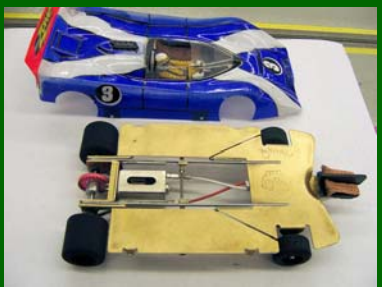
The Winning Car Tony P frame, 116.6 grams, JK T122, Red Fox Guide, JK Treated Rears, JK Fronts, 3rd Eye Controller
