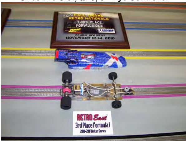
Matt's Car: Samson Chassis, O/S Chevron, 115.9 Grams, JK Fronts and Treated Rears, JK Guide, Fast Ones Pro Slot, 8/29, 3rd Eye Controller
