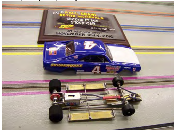
Randy's Car: Skunkworks Chassis, O/S Charger, 133.8 Grams, JK Wonder Rears, JK Fronts, Red Fox Guide, TSR, 9/28, 3 rd Eye Controller
