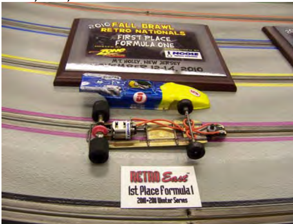
Matt's Car: Samson Chassis, O/S Chevron, 115.9 Grams, JK Fronts and Treated Rears, JK Guide, Fast Ones Pro Slot, 8/29, 3rd Eye Controller
