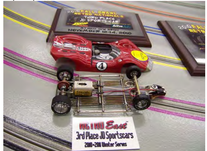
Mark's Car: Warmack Chassis, TSR Lotus 40, 115.3Grams, Pro Track Fronts and Rears, Jet Guide, F2, 8/28, Difalco Controller
