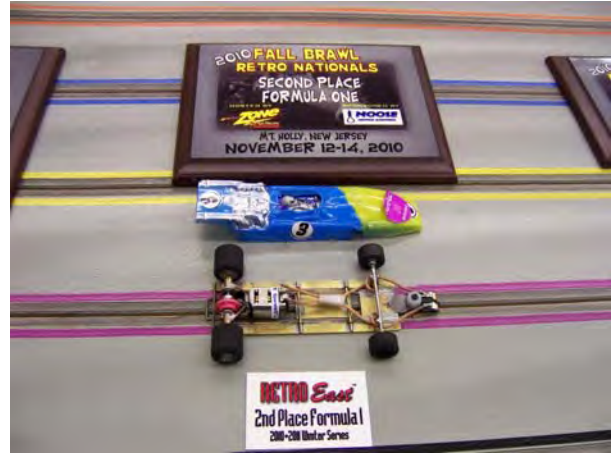
Mike's Car: Samson Chassis, O/S Chevron, 110.4 Grams, JK Fronts and Treated Rears, Parma Guide, Pro Slot, 8/30, Difalco Controller
