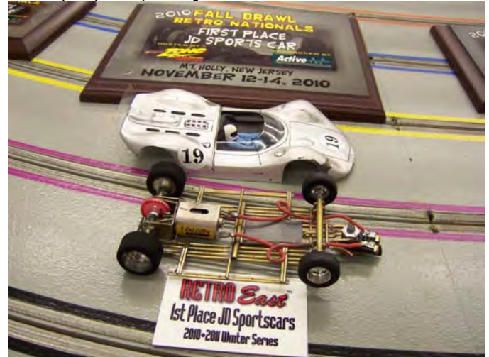
Howie's Car: Warmack Chassis, TSR Lotus 40, 115.3Grams, Pro Track Fronts and Rears, Red Fox Guide, F2, 8/28, 3 rd Eye Controller
