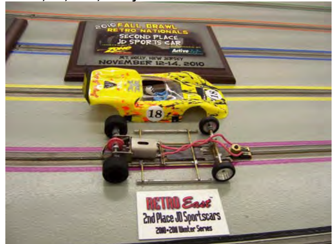
Mark's Car: Warmack Chassis, TSR Lotus 40, 115.3Grams, Pro Track Fronts and Rears, Jet Guide, F2, 8/28, Difalco Controller
