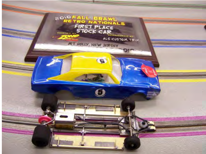
Mike's Car: Iles Chassis, O/S Charger, 133.8 Grams, JK Fronts and Rears, JK Guide, F7, 8/27 – Ruddock Controller
